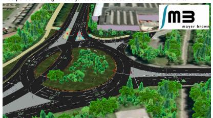
12d Model was used to design the layout so that the proposal could be constructed accurately. The need to adhere to the UK's 'DMRB' K-values meant that the vertical design became 'somewhat challenging', as they had to tie in with existing roads, drainage, and crossfalls, while maintaining a design path that complied with the standards, without compromising the efficiency of the layout.
