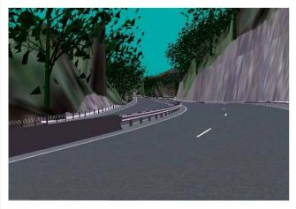
The concept design of the new highway was done in 12d and the bridges modelled using super strings. Roadside barriers and vegetation were also modelled in 12d to give a
