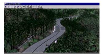
The original terrain was constructed from laser airborne scanning (LIDAR data) from a helicopter and then aerial photos were draped over the resulting triangulation to realistically represent the existing scene.
