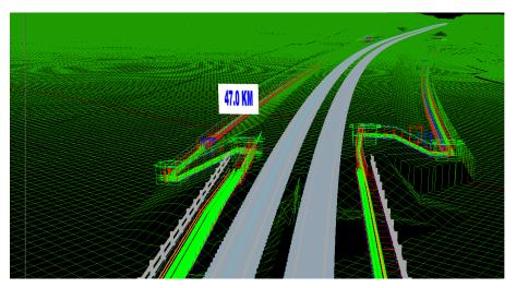
alignment with chainage generally corresponding to the pit locations. Any changes in length of the CSR and pit location require the chainage value in the MTF to be updated. Manually updating chainage in the MTF is very time consuming. A self-updating chainage MTF is required.
