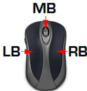
The left button is the ‘Select’ button – typically used to select graphic items or text. The middle button (or wheel) is the ‘Accept’ button, used to confirm a selection. The right button is the ‘Menu’ button. It is context sensitive and often displays a list of alternatives available at that instant.
