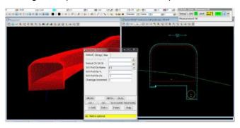
excavated surface and the design surface. Tunnels can be created normal to alignments or vertically using both plan and true, 3d chainages.
