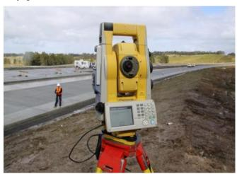
Surveyors and engineers are able to view and control Motorised Total Stations from the Tablet PC or view live GNSS on screen position whilst surveying.
