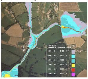
Users of the module can completely take advantage of 12d Model's ability to easily handle large datasets (including TINS and LIDAR). 12d Models 1d dynamic drainage is easily integrated with the surface flows.
