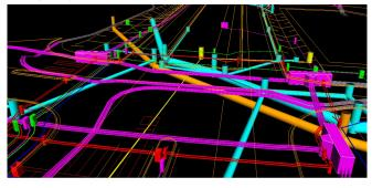
Users can design a complete drainage network and increase design quality through a holistic handling of design surfaces, other services, clash checking and trench quantities.
